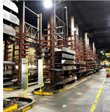
VIEW OF CANTILEVER RACKING
