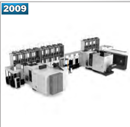
2009 MAZAK HORIZONTAL MACHINING CELL CONSISTING OF (2) MAZAK HCN-6800-II CNC HORIZONTAL MACHINING CENTERS
