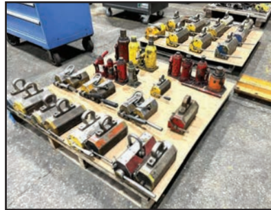
VIEW OF LIFTING MAGNETS
