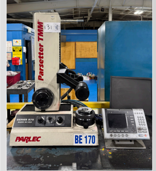
PARLEC PARSETTER TMM SERIES 975 TOOL PRESETTER
