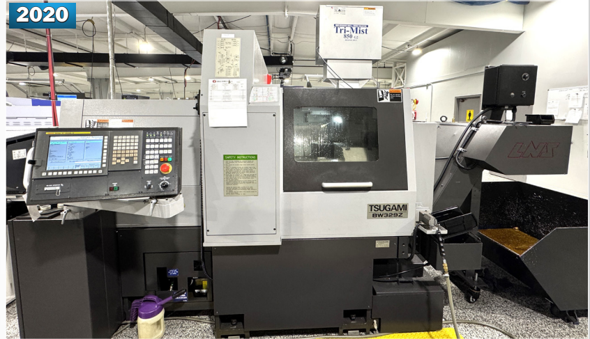
TSUGAMI BW-329Z CNC PRECISION SWISS TYPE LATHE
