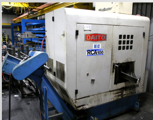
DAITO MODEL RCA 100 CIRCULAR COLD SAW
