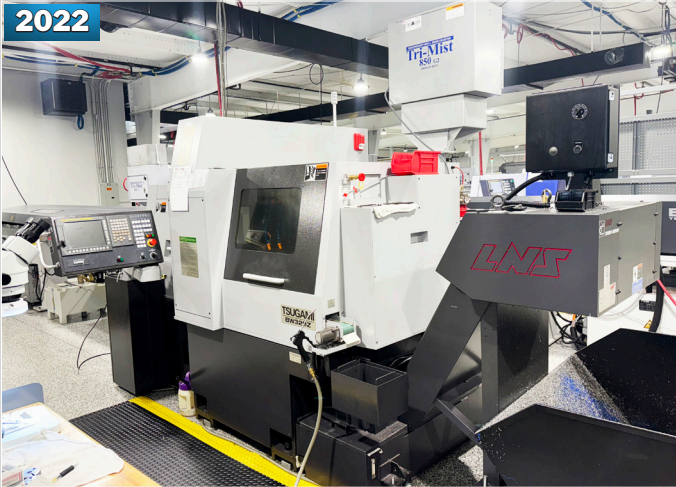
TSUGAMI BW-329Z CNC PRECISION SWISS TYPE LATHE
