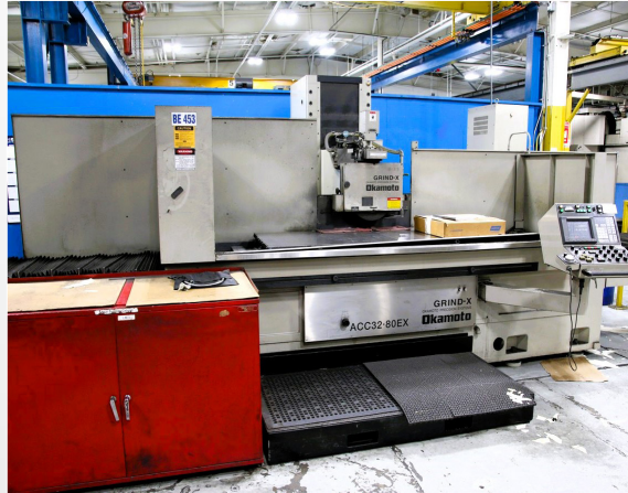
OKAMOTO ACC32-80EX 32" X 80" CNC HORIZONTAL SURFACE GRINDER
