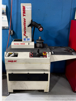
PARLEC PARSETTER TMM SERIES 1000 TOOL PRESETTER
