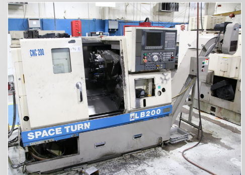
OKUMA SPACE TURN LB200 CNC SLANT BED LATHE
