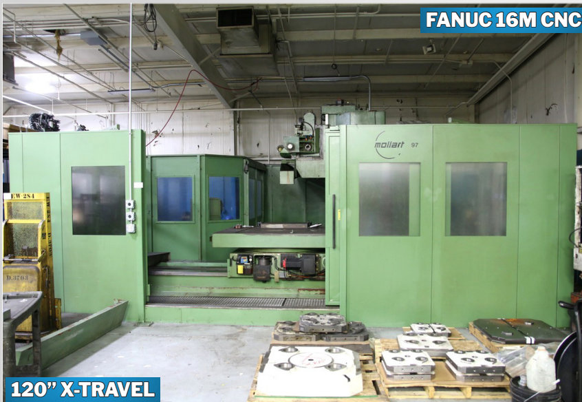
MOLLART PRISMABORE PRB3000 CNC GUN DRILL
