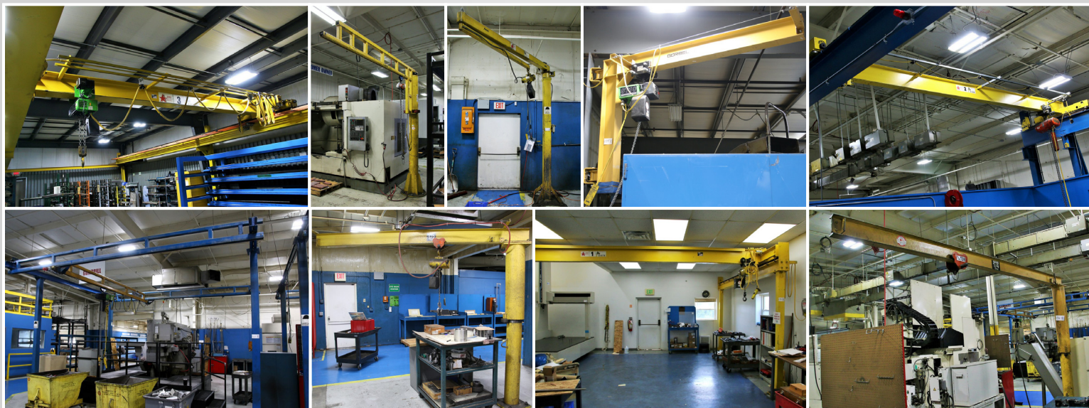
OVERHEAD BRIDGE CRANES, FLOOR-MOUNTED CRANE SYSTEMS, & JIB CRANES UP TO 5000 LB CAPACITY
